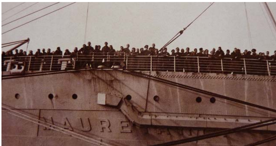
Figure 134: Troops crowded on to the MAURETANIA 's foredeck. Note the 'de-gaussing' cable, which neutralized the ship's magnetic field, and so helped in stopping magnetic mines being attracted to the ship (Liverpool Museums, UK)
