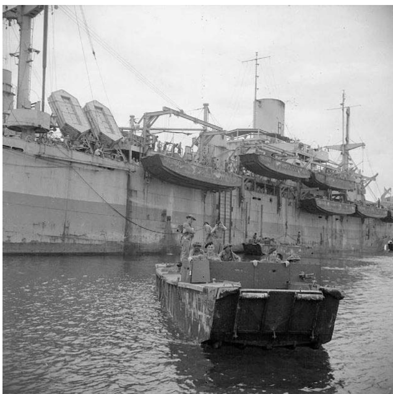
Figure 244: An LCA leaving the LSI HMS Rocksand for the island of Nancowry, on the Nicobar Islands, October 1945. Other LCAs are suspended on davits waiting to be loaded before being lowered.
