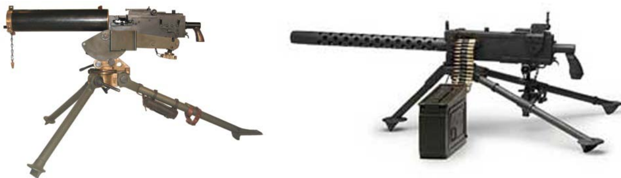
Figure 40: M1917 Water-cooled heavy machine gun (left) and M1919A Air cooled light machine gun (right) – Public Domain
